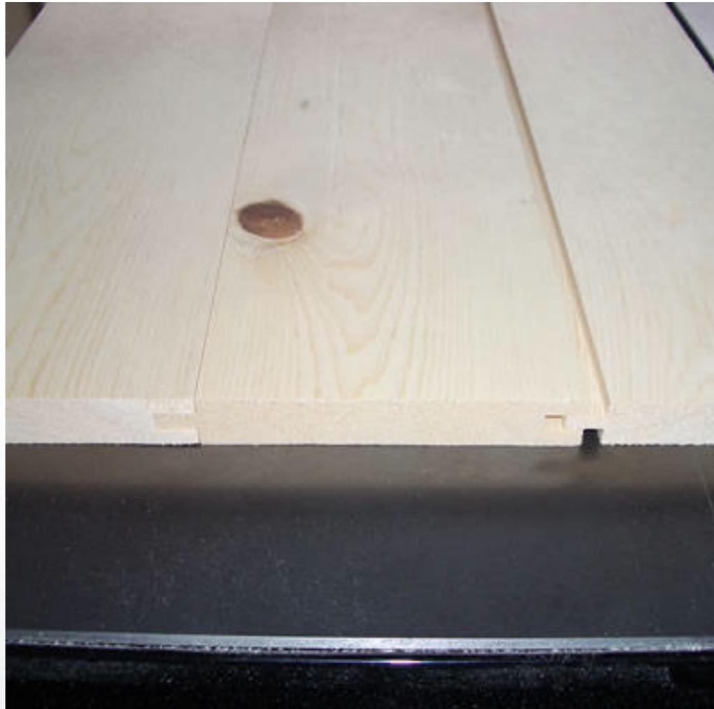
When joining two boards along a long edge, one can simply butt the joint together and hold it with glue. However, the tongue and groove joint is stronger and provides more glue surface. Learn how to create consistent tongue and groove joints.
