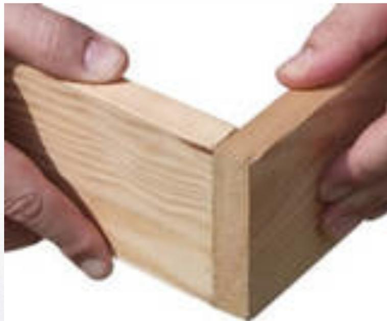
The butt joint is the most basic woodworking joint. Commonly used when framing walls in conventional, stick-framed homes, this joint relies on mechanical fasteners to hold the two pieces of stock in place. Learn how to build a proper butt joint, and when to use it on your woodworking projects.
