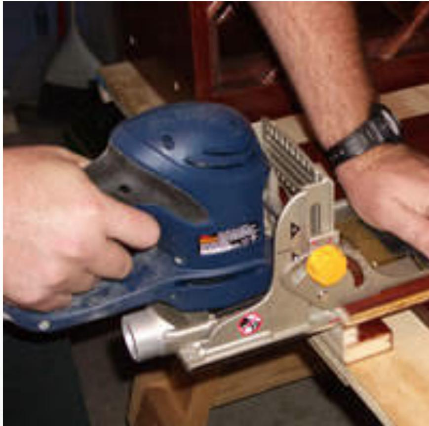
Another method for joining boards along the edges (like the tongue and groove joint) is to cut slots and use beechwood biscuits to hold the boards in place. This is a very common modern woodworking joint, relying on glue and the swelling of the beechwood biscuit to hold the boards in place. Learn how to cut consistent slots and get reliable results from biscuit joinery.
